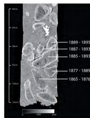
Figure1: CT scan of a back-reef sediment core with U-series ages in stratigraphic sequence.
